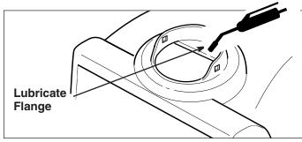
Figure 11. Grease the Discharge Chute Ring
